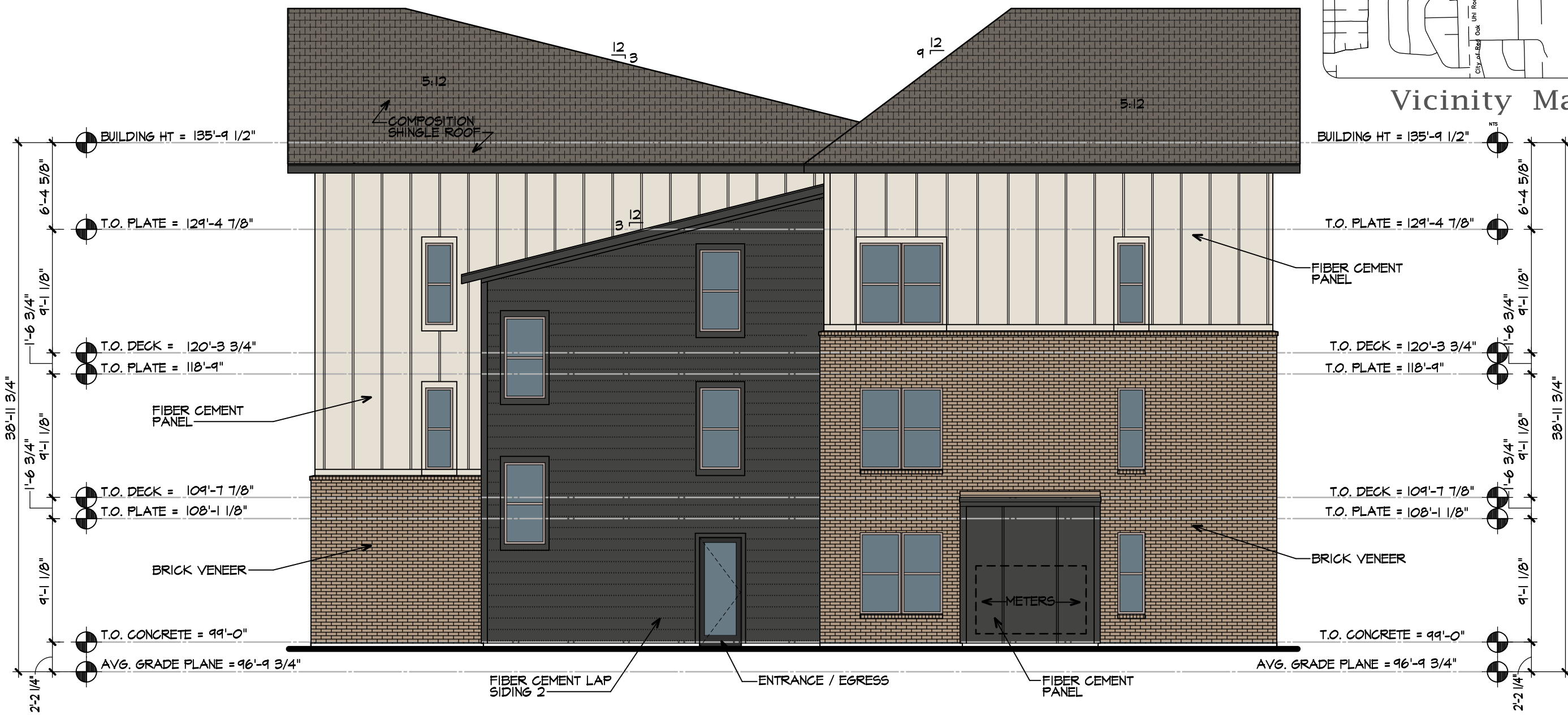
02 LEFT ELEVATION BUILDING #8 SCALE: 1/8"=1'-0"
