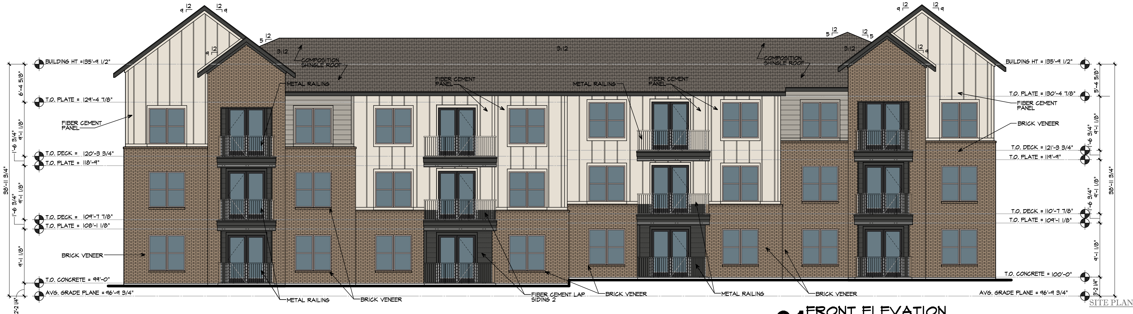
01 FRONT ELEVATION BUILDING #8 SCALE: 1/8"=1'-0"
